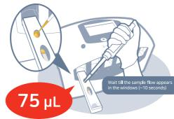
Insert a cartridge into i-chamber and incubate for 12 minutes
