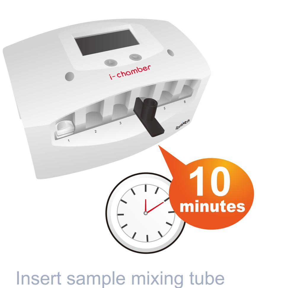
into the inserting tube block. Wait for 10min.
