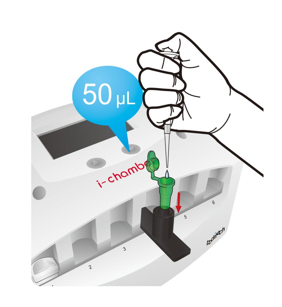
Transfer 50uL of releasing buffer into Sample mixing tube
