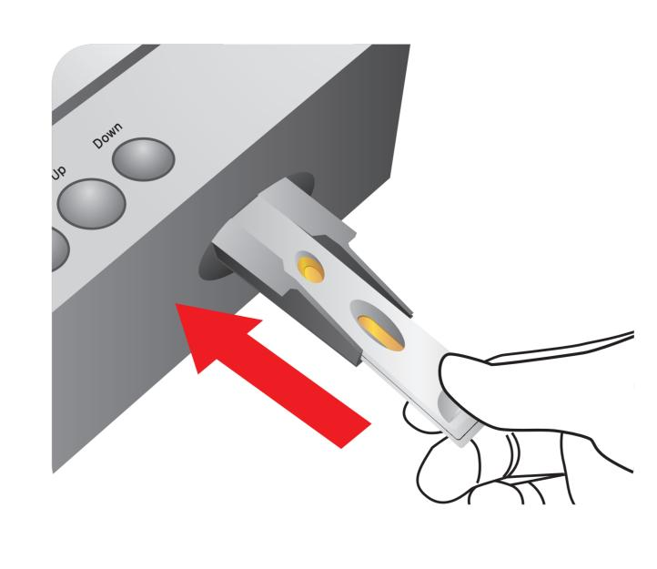
Insert the test cartridge into ichroma reader and press 'SELECT' button
