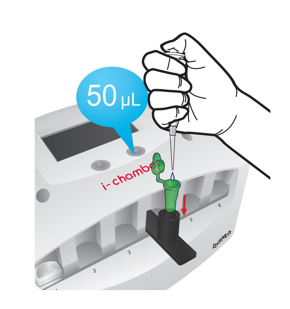
Transfer 50uL of releasing buffer into Sample mixing tube
