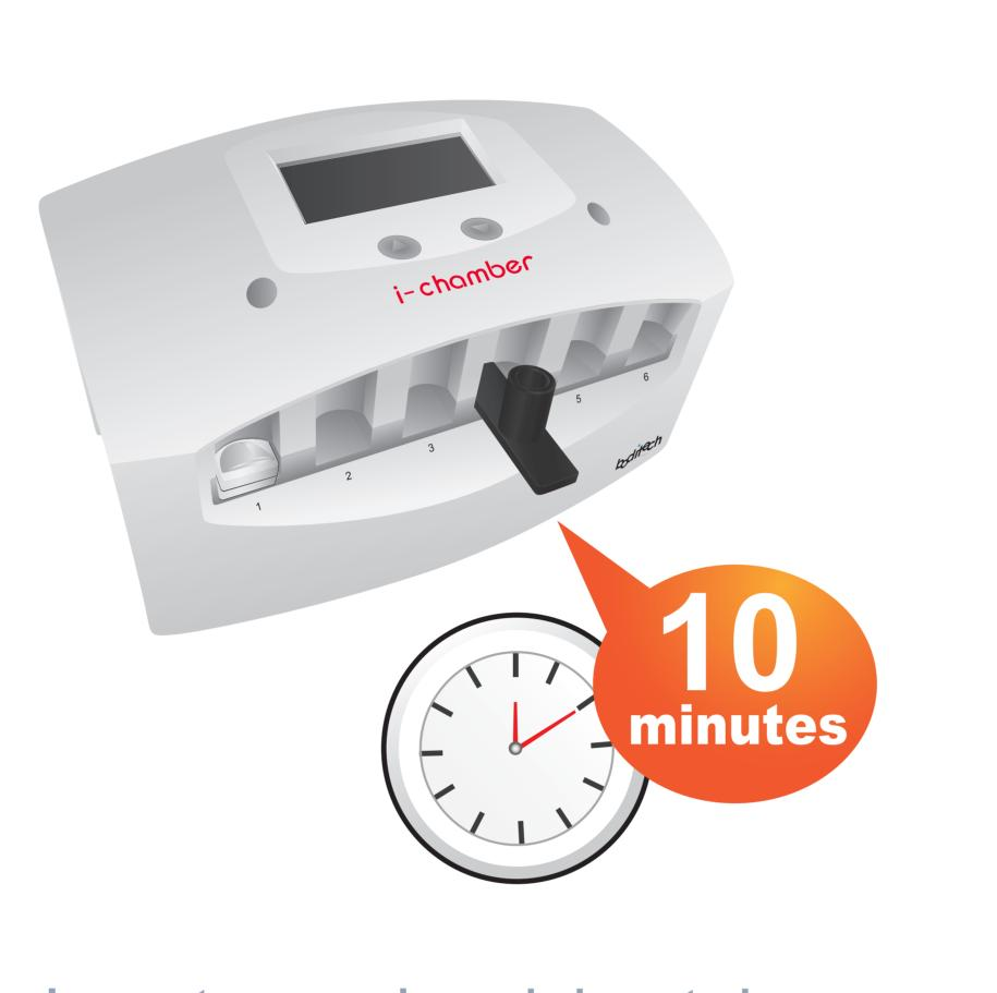
Insert sample mixing tube into the inserting tube block. Wait for 10min.
