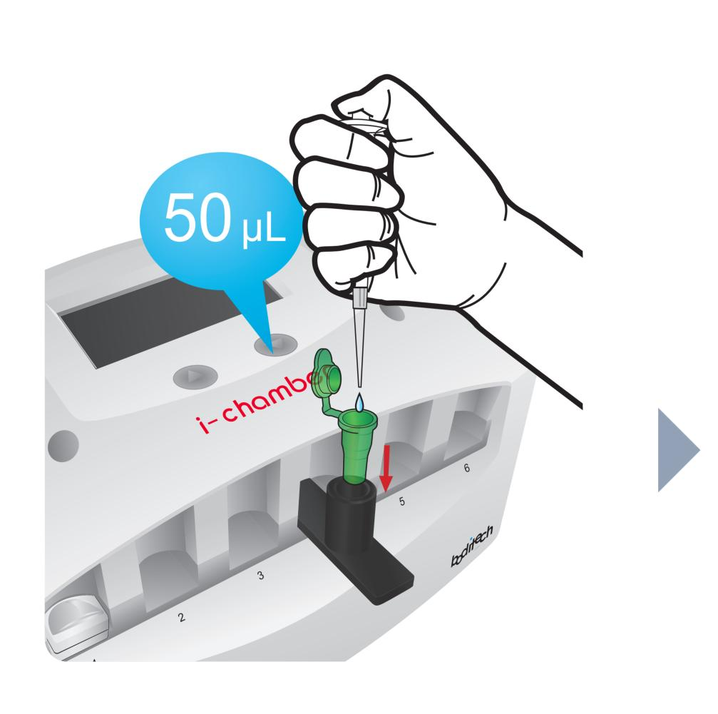
Add 50uL of sample into Sample mixing tube.
